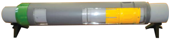
图 5 套管固井试油压裂滑套 3D 打印模型 Fig.5 3D printing model of cased hole testing fracturing sliding sleeve
