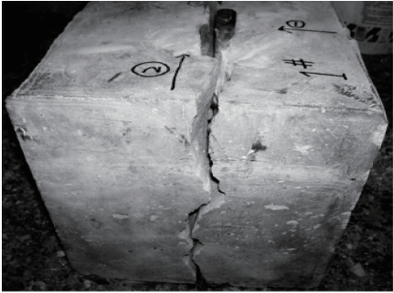
图 4 大型岩样人工裂缝形态 Fig.4 Artificial fracture morphology in large-scale rock sample
