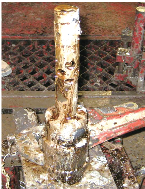
图5 点火头上沉积的重晶石粉和泥砂实物图 Fig.5 Barite powder and silt deposits deposited on the ignition head
