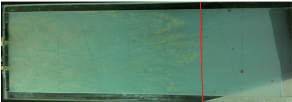
图 2 连续加砂方式下的支撑裂缝铺置形态 Fig.2 Placement pattern of supporting fractures under continuous sanding
