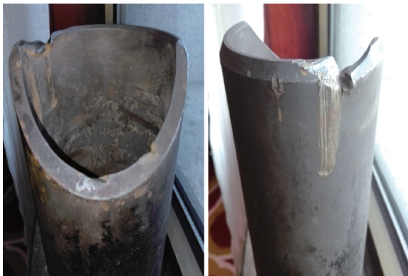
图 3 回接管端部错口损伤实物图 Fig.3 Physical drawing of wrong mouth damage at the end of back intubation
