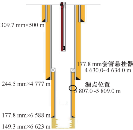
图 4 TP1’井井身结构示意图 Fig.4 Schematic diagram of well bore structure of Well TP1’
