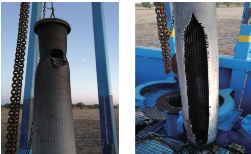
图 4 压差过大造成砂筒撕裂实物图 Fig.4 Physical picture of sand cylindr tornd by too large pressure difference
