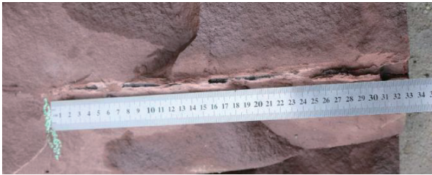
图 4 高钨粉药型罩穿砂岩靶孔道效果图 Fig. 4 Design sketch of high tungsten powder liner penetrating sandstone target channel
