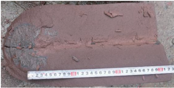
图 5 活性药型罩穿砂岩靶孔道效果图 Fig. 5 Design sketch of active charge liner through sandstone target channel
