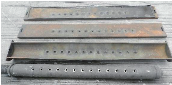
图 5 射孔后的背托、盖板、178 mm 套管 Fig. 5 back support, cover plate and 178 mm casing after perforation
