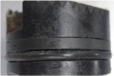
图 4 RPTFE 材料背圈耐温压测试结果 Fig. 4 Temperature and pressure test results of RPTFE back ring
