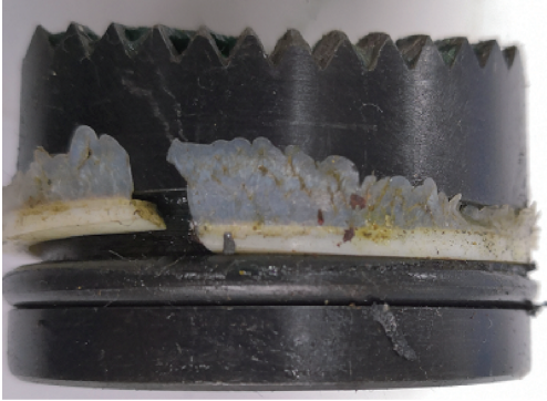
图 3 PTFE-F4 材料背圈耐温压测试结果 Fig. 3 Temperature and pressure test results of PTFE-F4 back ring
