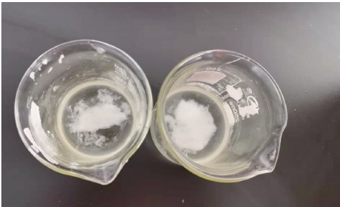
图 3 实验 2(左)和实验 7(右)冻胶压裂液破胶效果图 Fig. 3 Experiment 2 (left) and Experiment 7 (right) gel breaking effect diagram of gel fracturing fluid
