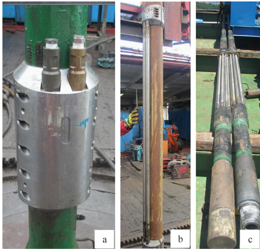
图 4 中继器与井下压力计连接图 Fig. 4 Connection method of repeater and downhole pressure gauge
