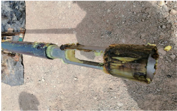
图 1 D11 井通井工具串带出蜡样现场照片 Fig.1 The D11 well pass tool string brings out the wax sample site photos
