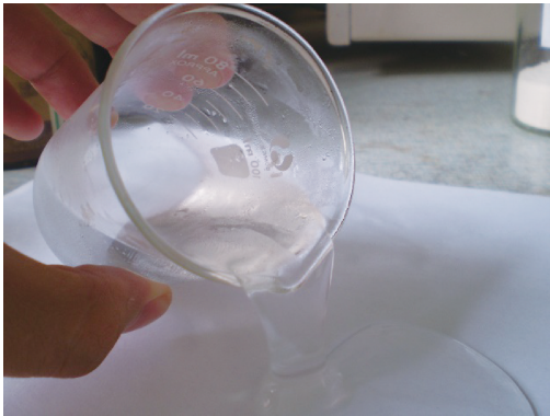
图 2 无水改性乙二醇基速溶压裂液在-19 ℃的状态 Fig. 2 Anhydrous modified glycol based instant fracturing fluid at -19 ℃
