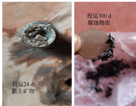
图2 A井投运后不同阶段堵塞物质分析 Fig. 2 Analysis of blockage substances at different stages after the operation of well A
